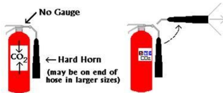
The pressure in a CO<sub>2</sub> extinguisher is so great; bits of dry ice might shoot out of the horn!
